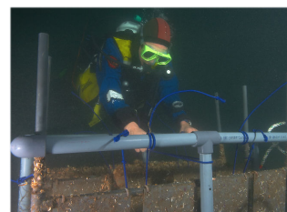
Sub-surface recovery of settlement panels
